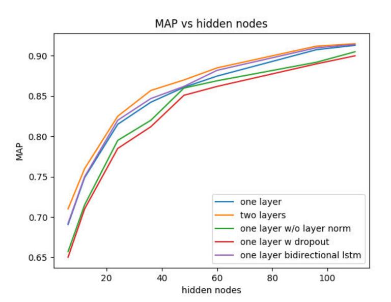
• Different versions of the model are tried with increasing number of hidden nodes and its noted that a single layer with layer norm provides the best tradeoff with respect to the parameters and MAP
